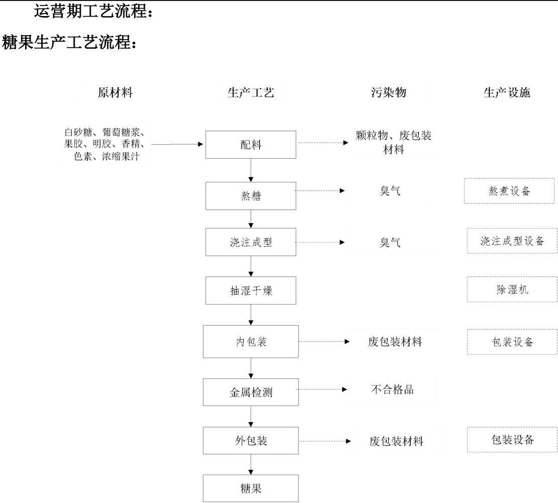
图 2-3 糖果生产工艺流程及产污环节图
